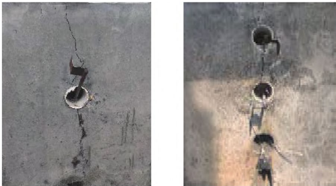
Figure 1.7 Specimen surface damage pattern (Xiao et al. 2022)
